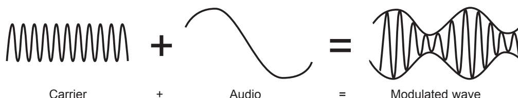
Fig 1-6: Carrier wave plus AM wave form
