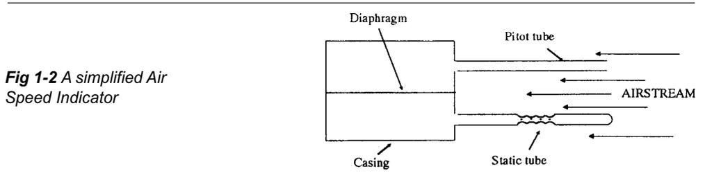
**Fig 1-2** A simplified Air Speed Indicator
