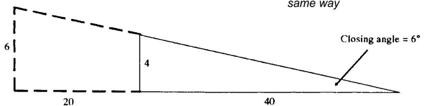
11. Once you understand the method and can do the mental arithmetic, you can then omit the drawing of the triangles in Figs 3-4 and 3-5. Putting these figures back into the original problem from Fig 3-3, you can see that the track error angle and the closing angle are added together to give  $18^\circ$ , this is the amount that you need to turn right in order to regain track at point B.
