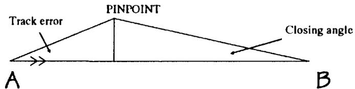
4. An aircraft flying from A to B finds that after 30 nm it is 4 nm off track. If it has a further 60 nm to travel by how much does the pilot need to turn to regain the intended track at B?
