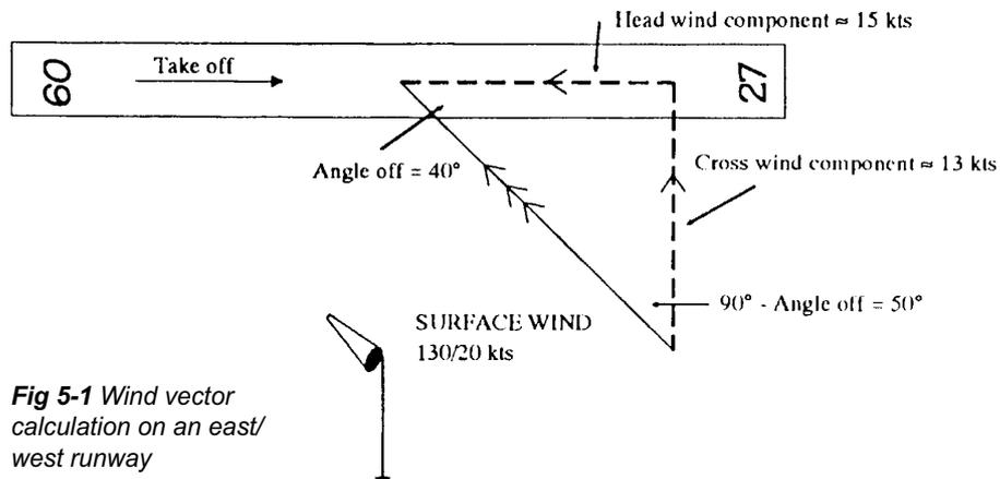
**Fig 5-1** Wind vector calculation on an east/west runway
