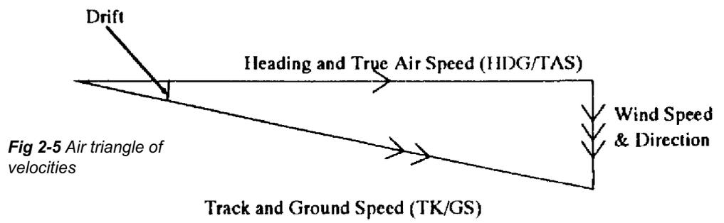
*Fig 2-5 Air triangle of velocities*
