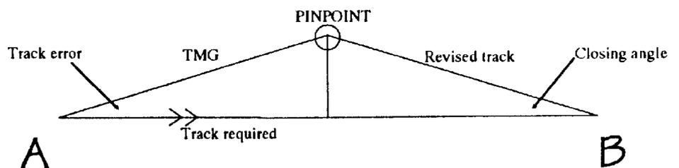
8. As the triangles are the same size and shape, it is only necessary to alter heading to the right by twice the track error to ensure that the aircraft reaches point B (assuming that the wind remains constant). As the pinpoint is taken halfway along track, the actual distances do not affect the results, but in the next example the only pinpoint available is one third of the way along track so some sums are needed.
