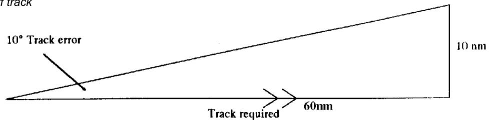
6. The 1 in 60 rule holds good for track errors up to 23° beyond that the difference in the length of the two tracks (TMG and Track required) becomes too great and the approximation will not work.
